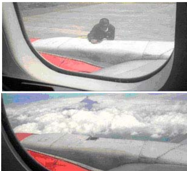
An Adam Air instant airframe tape patch, emblematic of the type of maintenance witnessed by passengers. The tape was used to hold down a panel that was reluctant to stay closed on the 737 engine support fairing. As shown in the photograph below, the tape is starting to lift. This type of cell phone photograph taken by a passenger is increasingly likely to find its way onto the Internet.
